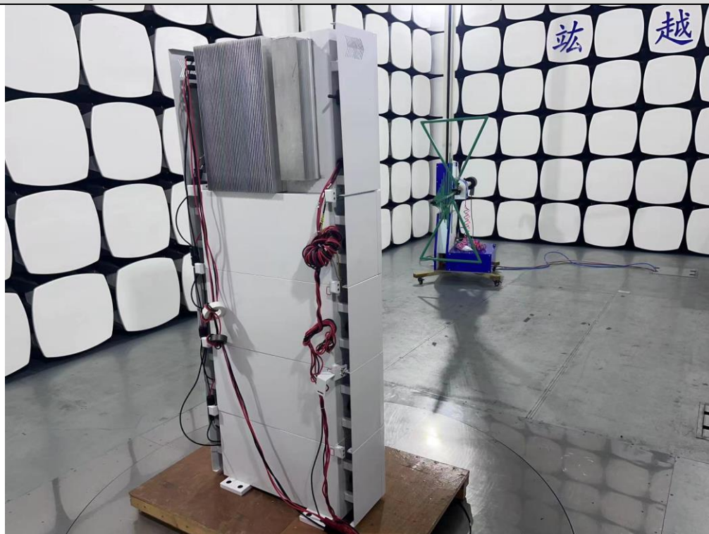
Radiated electromagnetic disturbances (30 MHz to 1000 MHz):Back View
